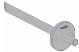
3 Connect the hose between the pressure outlet and the pressure switch's nipple, as shown. This point is important for correct functioning. The pressure switch "-" connector must not be used.
